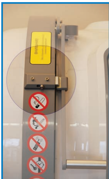
The construction of the hyperbaric chamber has a locking device on the cover
